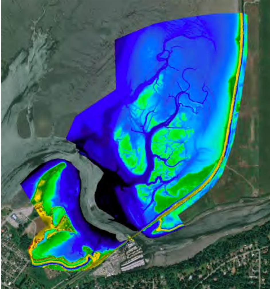
Figure 19 Colourized Nicomeckl Digital Elevation Model (DEM) for October 2018 overlain on a satellite image
