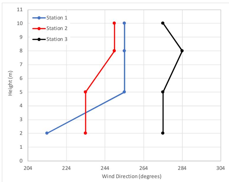
**Figure 3-6** Wind direction profiles during a moderate wind event on 25 October 2019, collected adjacent to the Colebrook Road Pump Station (station 1) and 110 m and 270 m west along the dyke road from the pump station (station 2 and 3 respectively).
