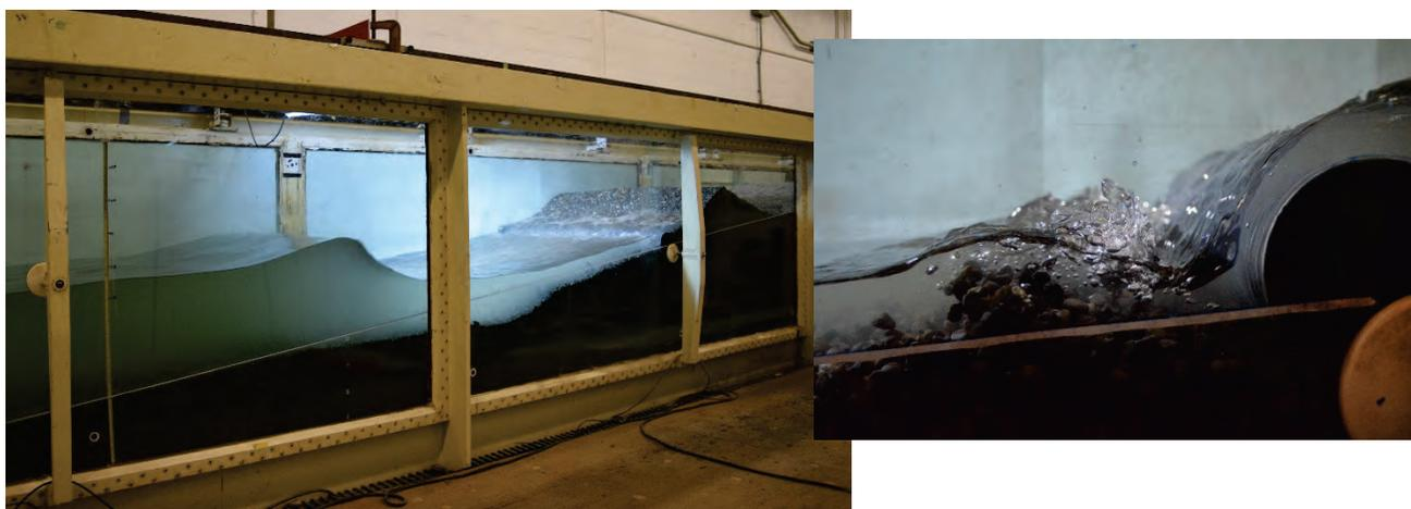
Figure 3.3 Photos of physical model studies undertaken by J. Wilson of the effects of woody debris on shoreline response during storm events at the National Research Council, Fall 2019 (J. Wilson, NHC)
