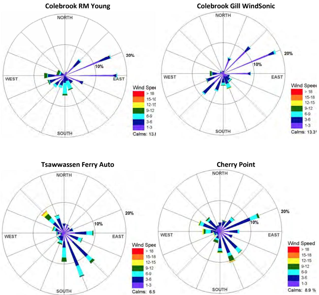
**Figure 3-8** Wind rose frequency distributions, given in percent occurrence, at Colebrook Road Pump House Onshore Wind Monitoring Station and selected proximate stations based on available wind speed and direction data during the 1 September to 31 October 2019 preliminary assessment period.
