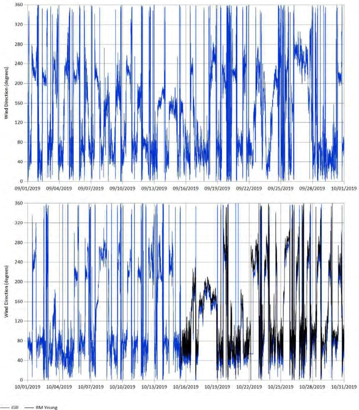
**Figure 3-3** Wind direction data during the 1 September to 31 October 2019 preliminary assessment period from the RM Young mechanical and Gill WindSonic ultrasonic wind sensors installed at the Colebrook Road Pump House Onshore Wind Monitoring Station. Data are 2-minute average values based on 3 second samples.
