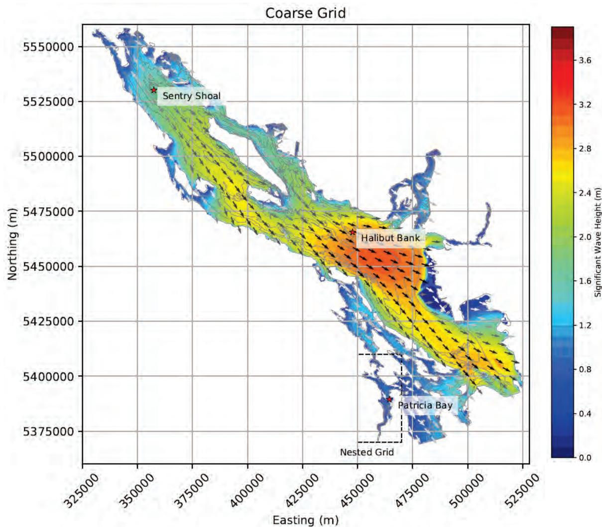
**Figure 2.1** An example of output from a phase averaged wave model (NHC, SWAN model), utilizing a spatially varying wind field developed using measured winds from airports, lighthouses, and wave buoys.
