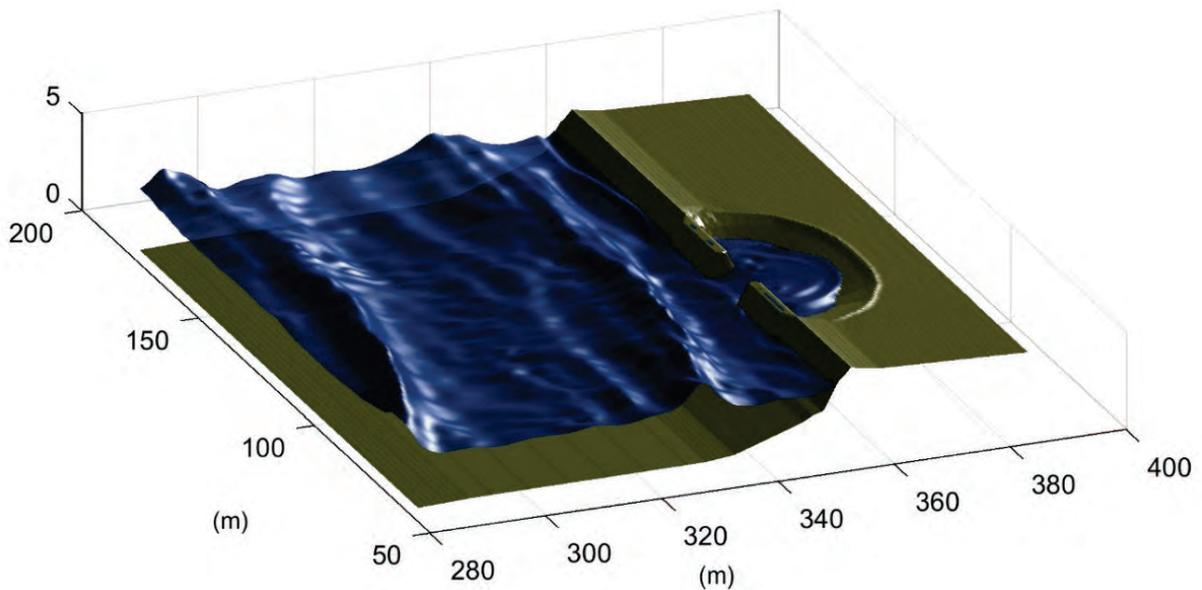
**Figure 2.2** An example of output from a phase resolving wave model (NHC, SWASH model), used to examine wave-structure interactions along a section of dike that has been opened to enhance ecological habitat (Vertical scale enhanced).
