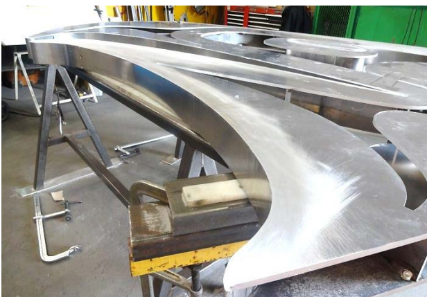
Finished to create a precise edge
