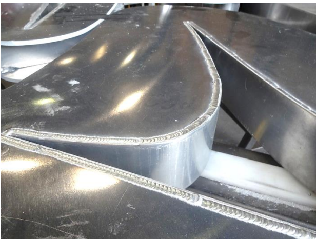
Walls welded to sheets creating 3D form
