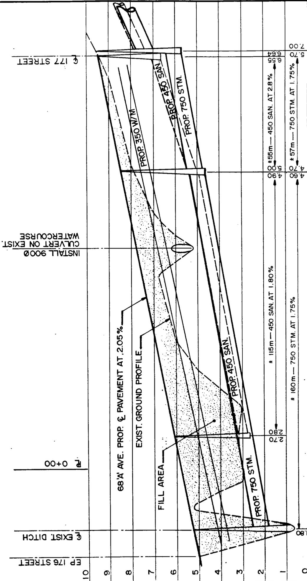
PRELIMINARY STORM, SANITARY & WATER PROFILES TO ACCOMMODATE 68' AVENUE CULVERT CROSSING
