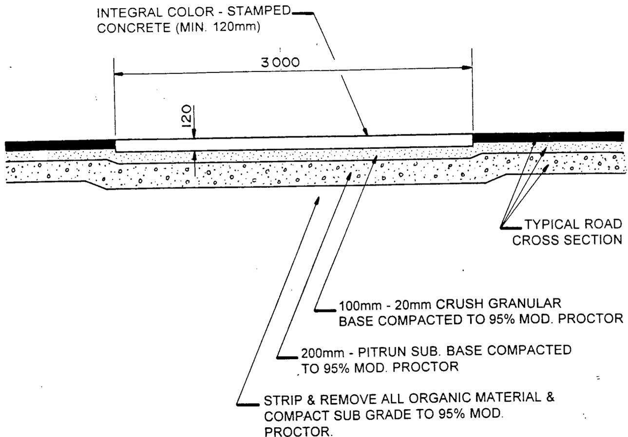
CONCRETE PAVEMENT CROSSING DETAIL
