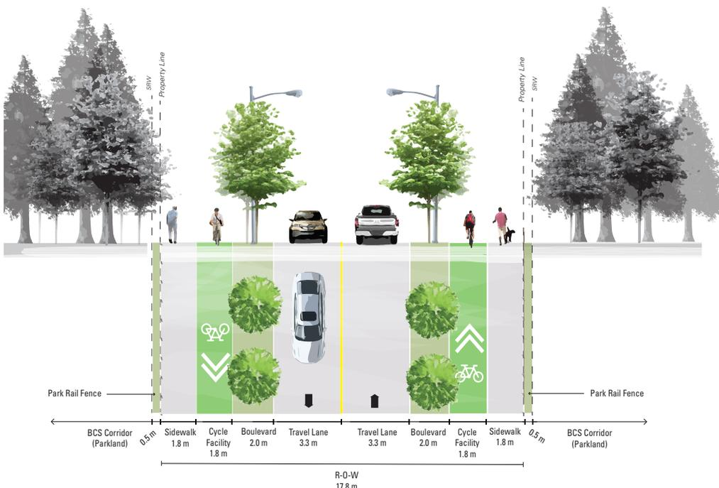
Figure 4.9 Collector BCS Road Crossing - 17.8 m Cross-section
