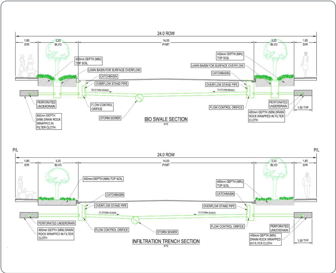
Figure 6.4 24 M Road Right-of-Way Bioswale & Infiltration Trench Cross-sections
