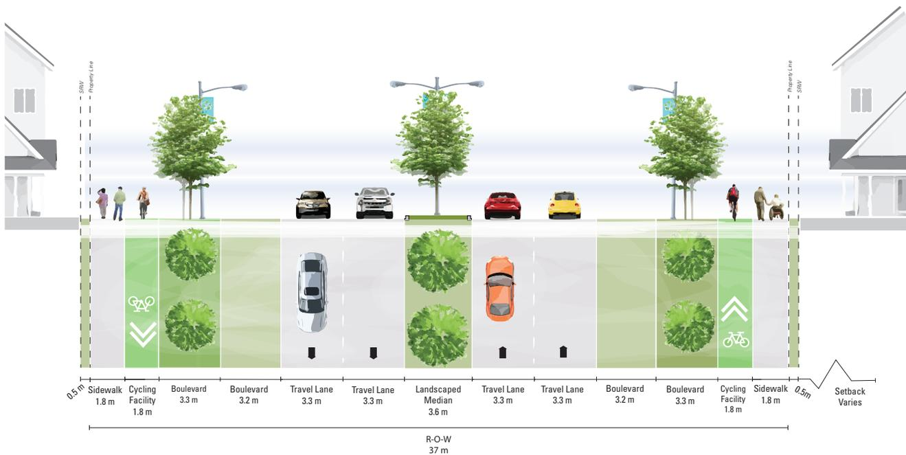
Figure 4.3 Arterial - 24 Avenue Interim 4 Travel Lanes (37 m Cross-section)
