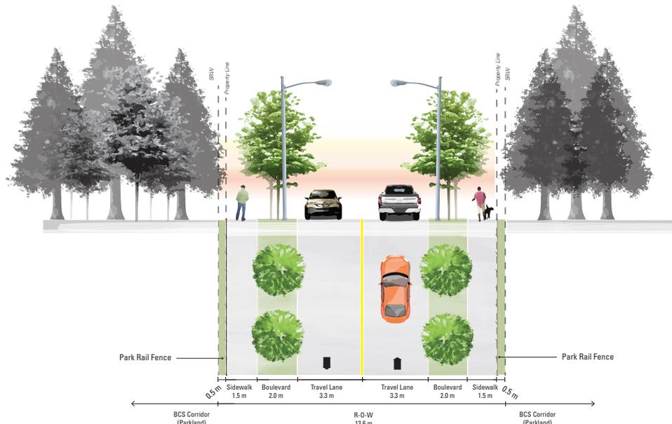
Figure 4.10 Local BCS Road Crossing 13.6 m Cross-section
