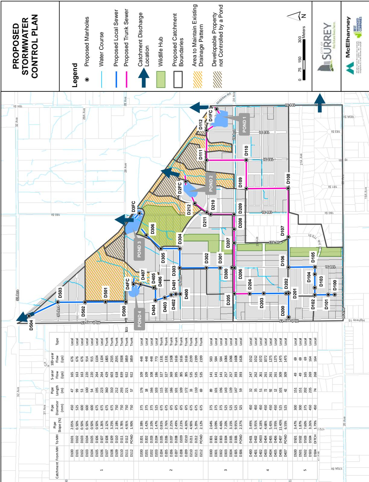
Figure 6.6 Proposed Storm Water Control Plan
