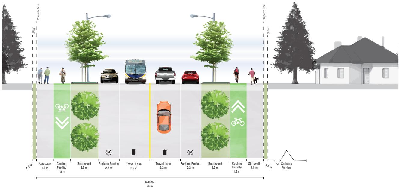
Figure 4.6 Standard Collector Road 24 m Cross-section
