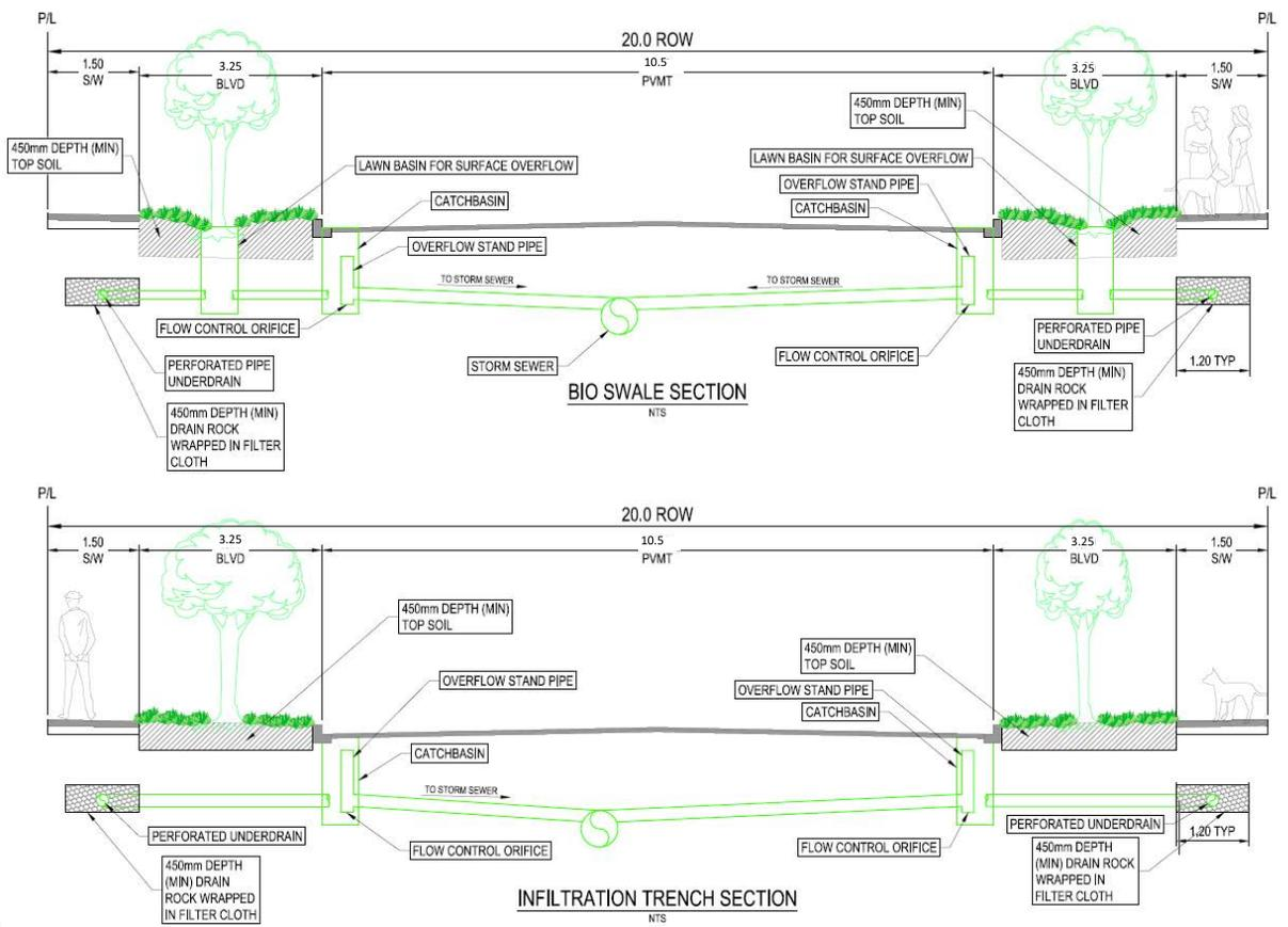
Figure 6.3 20 M Road Right-of-Way Bioswale & Infiltration Trench Cross-sections
