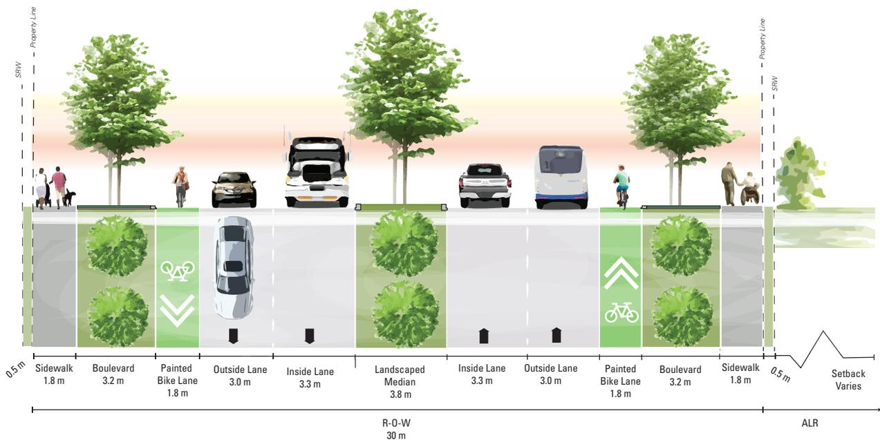
Figure 4.5 Arterial Standard - 32 Ave/184 St 30 m Cross-section
