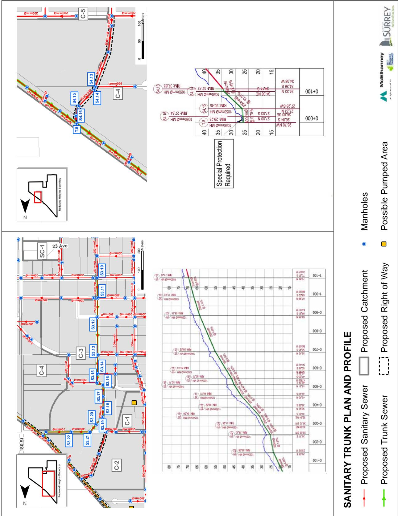
Figure 6.10 Sanitary Trunk Plan and Profile
