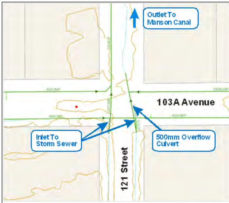
**Figure 4.3 - Conveyance Piping at Intersection of 121 St and 103A Avenue**
