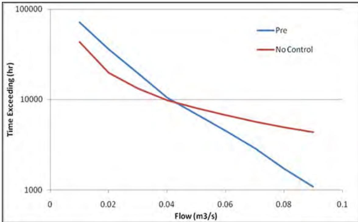
**Figure 2.19 – Flow Exceedance Curve for a Typical Pre-Development (Pre) and Post-Development with no BMPs or Ponds (No Controls)**
