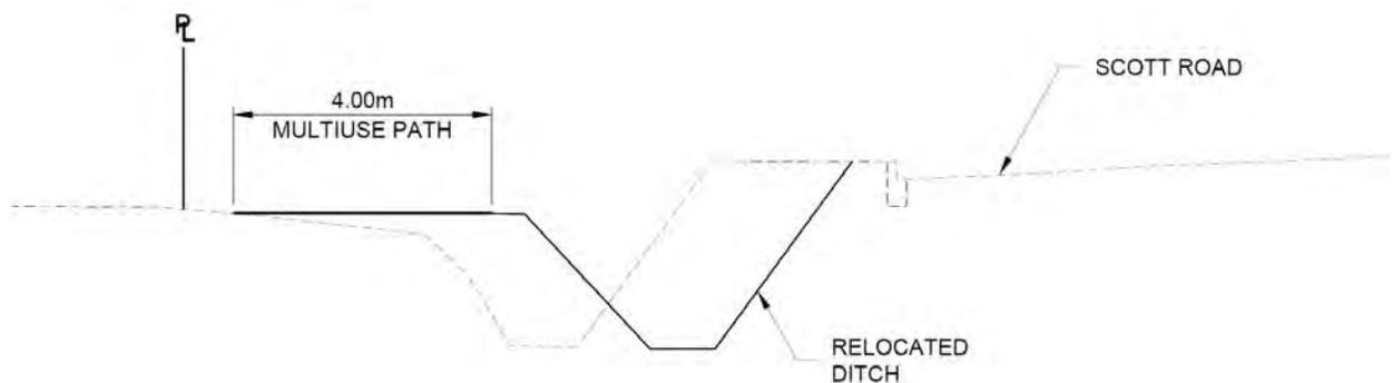
**Figure 3 - Schematic MUP Closer to Property Line**
