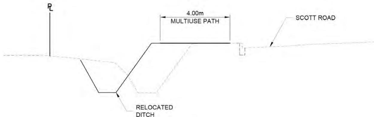
Figure 2 - Schematic MUP Closer to Scott Road
