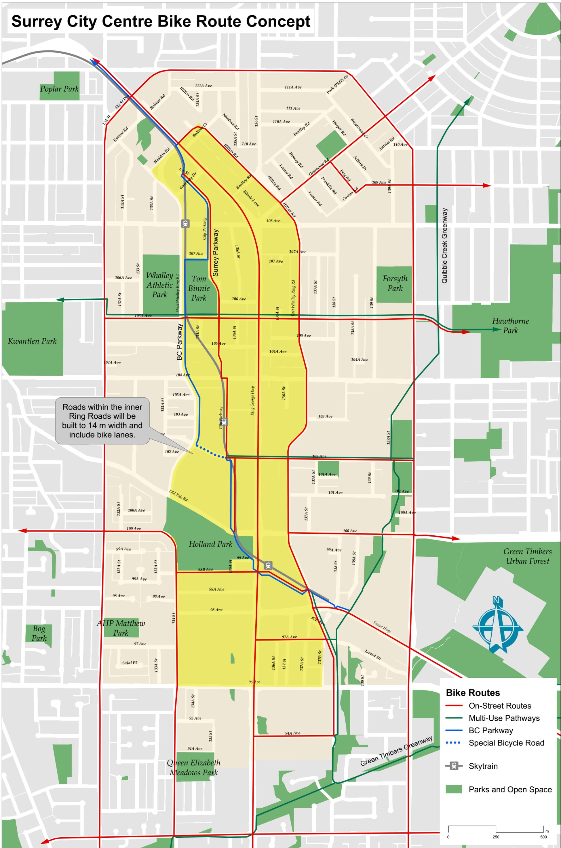
Roads within the inner Ring Roads will be built to 14 m width and include bike lanes.
