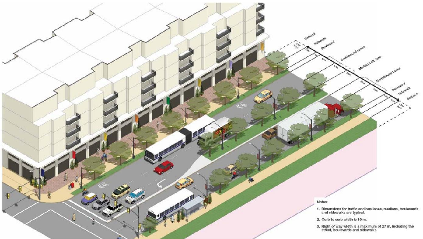
**Exhibit 6.4** is an illustration of a three-lane collector street with a left –turn lane at the intersection and parking along the curb elsewhere. This street would include medium-wide sidewalks, a landscaped boulevard with street trees, marked crosswalks, street lighting for both the traffic lanes and the sidewalks, and access to the parking spaces (and parking meters) from the sidewalk. Note that each of the curb lanes has exclusive bicycle lanes marked by continuous lines.
