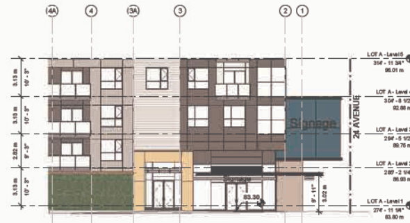
2 East Elevation (162 STREET) SIGNAGE (LEVEL 2) A402.A 1" = 10'-0"
