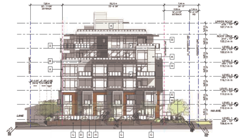
2 WEST ELEVATION (142 ST.) 3/32" = 1'-0"
