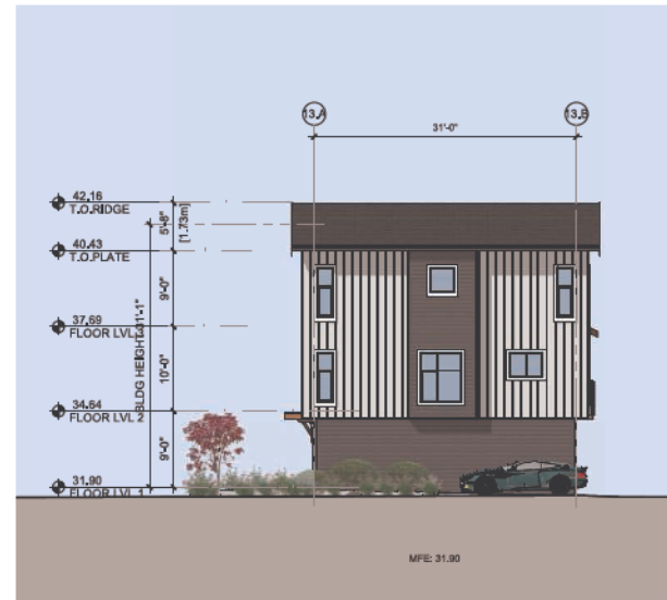
4 BUILDING13 - SOUTHWEST ELEVATION SCALE: 1/16" = 1'-0"
