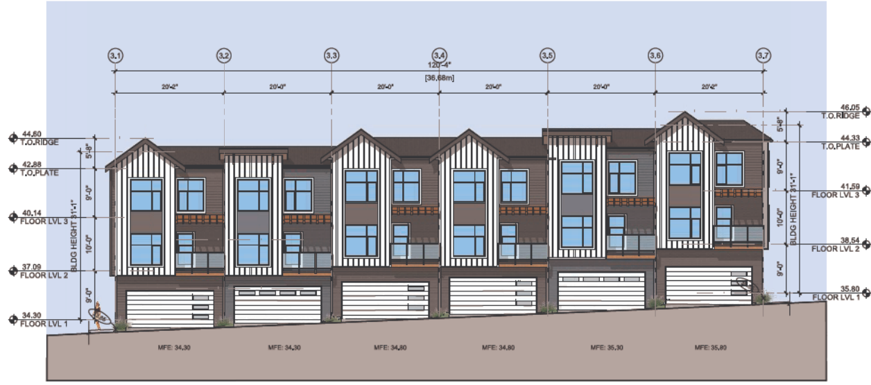
3 BUILDING3- WEST ELEVATION SCALE: 1/16" = 1'-0"
