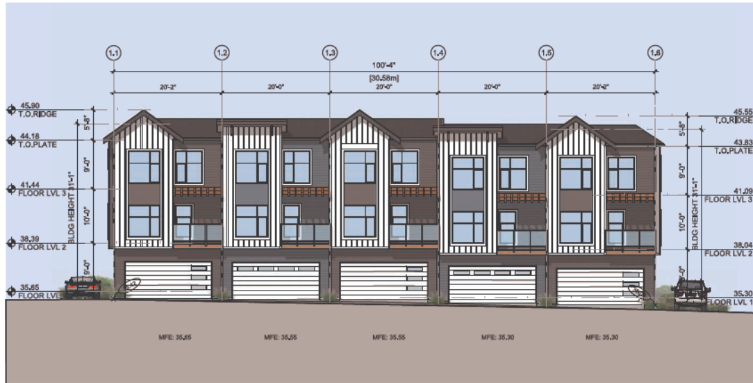
3 BUILDING1- NORTH ELEVATION SCALE: 1/16" = 1'-0"
