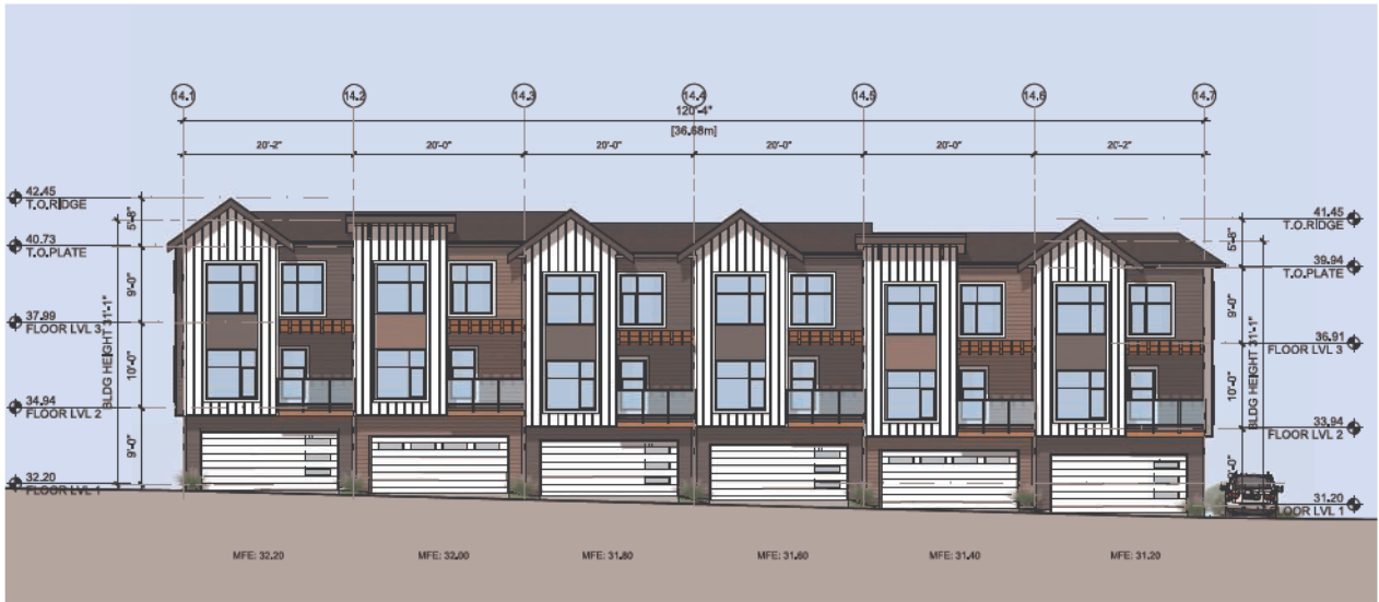
3 BUILDING 14 - EAST ELEVATION SCALE: 1/16" = 1'-0"
