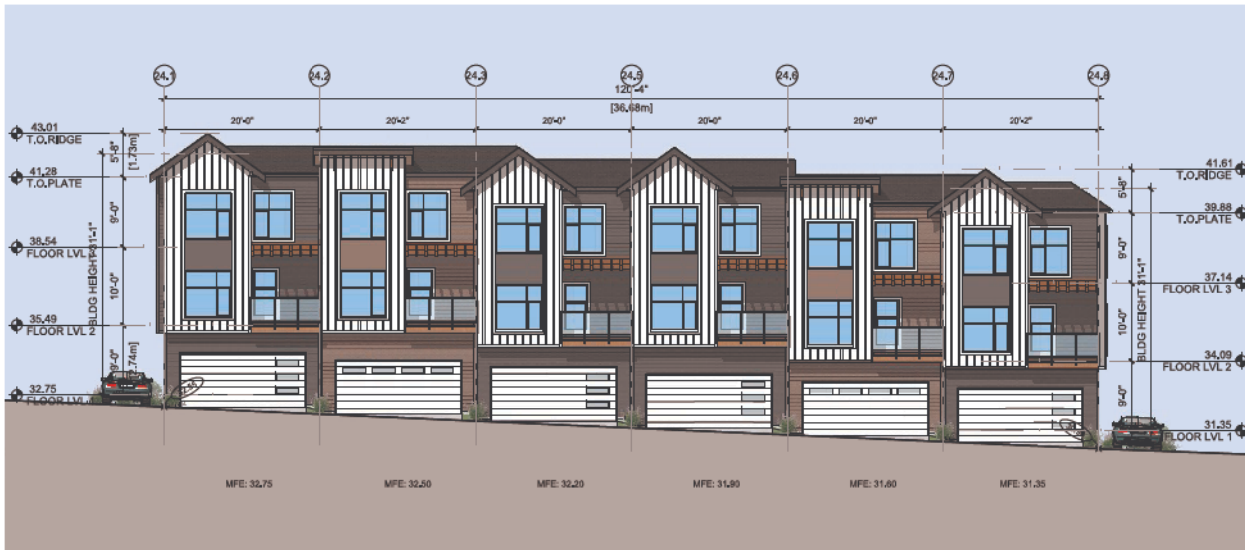
3 BUILDING24 - EAST ELEVATION SCALE: 1/16" = 1'-0"
