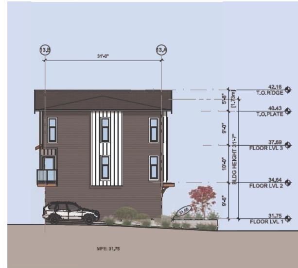
2 BUILDING13 - NORTHEAST ELEVATION SCALE: 1/16" = 1'-0"
