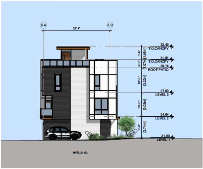
2 BUILDING 4- NORTH ELEVATION SCALE: 1/16" = 1'-0"
