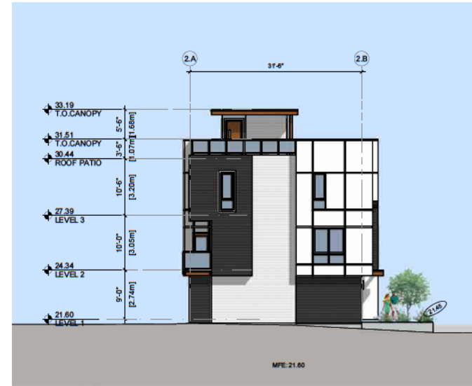
2 BUILDING 2- SOUTH ELEVATION SCALE: 1/16" = 1'-0"
