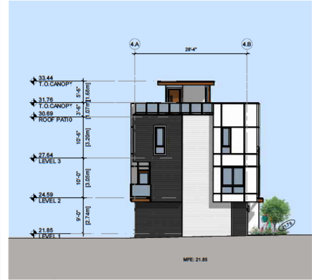
2 BUILDING 5- NORTH ELEVATION SCALE: 1/16" = 1'-0"
