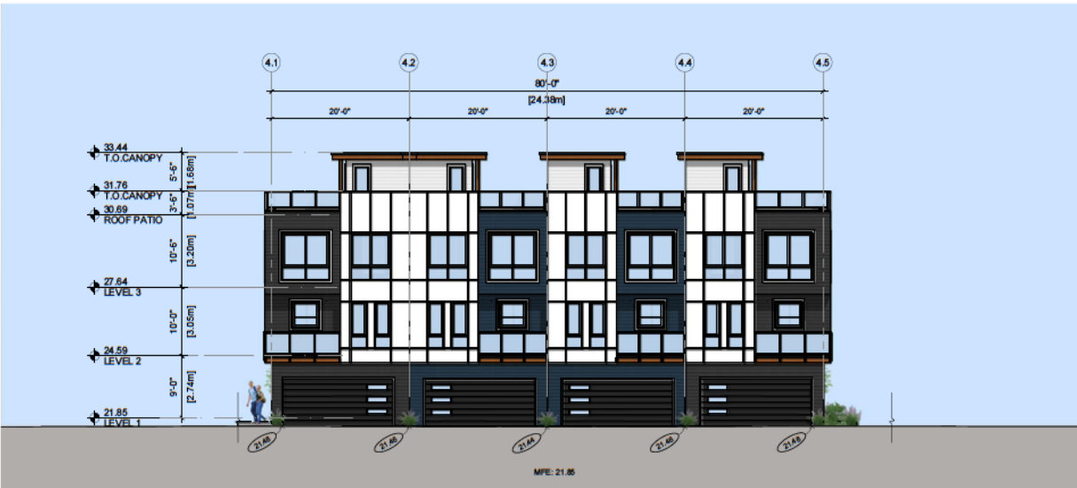
3 BUILDING 5- EAST ELEVATION SCALE: 1/16" = 1'-0"
