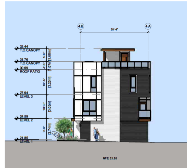
4 BUILDING 5- SOUTH ELEVATION SCALE: 1/16" = 1'-0"
