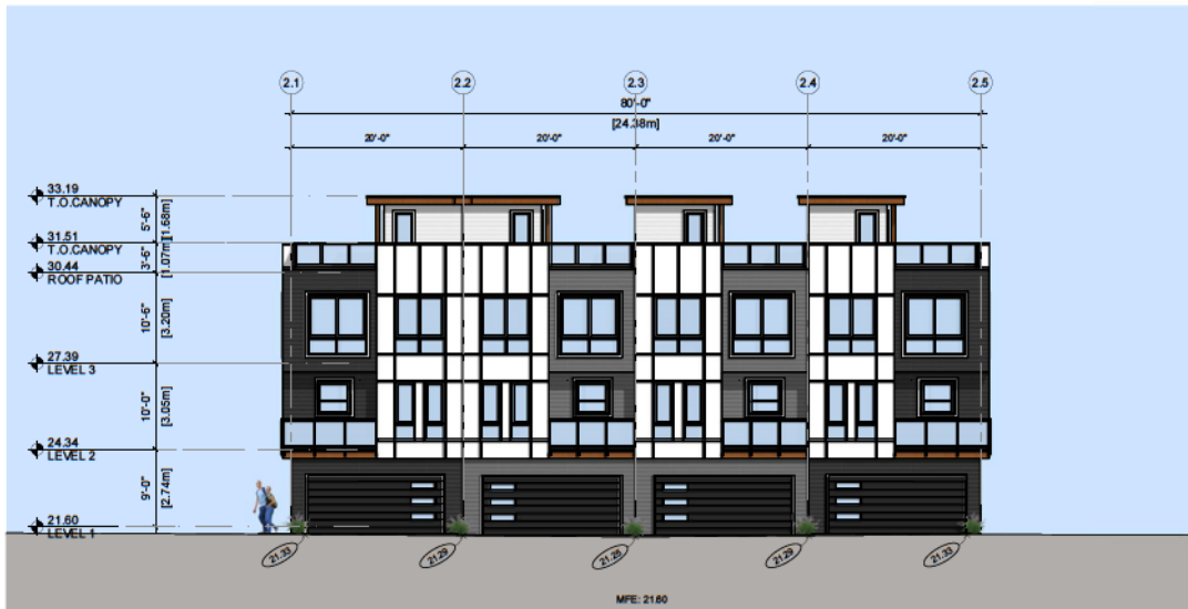
3 BUILDING 2- WEST ELEVATION SCALE: 1/16" = 1'-0"
