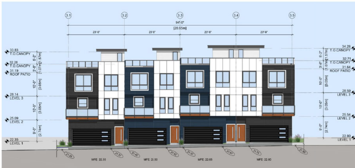
3 BUILDING 3- NORTH ELEVATION SCALE: 1/16" = 1'-0"
