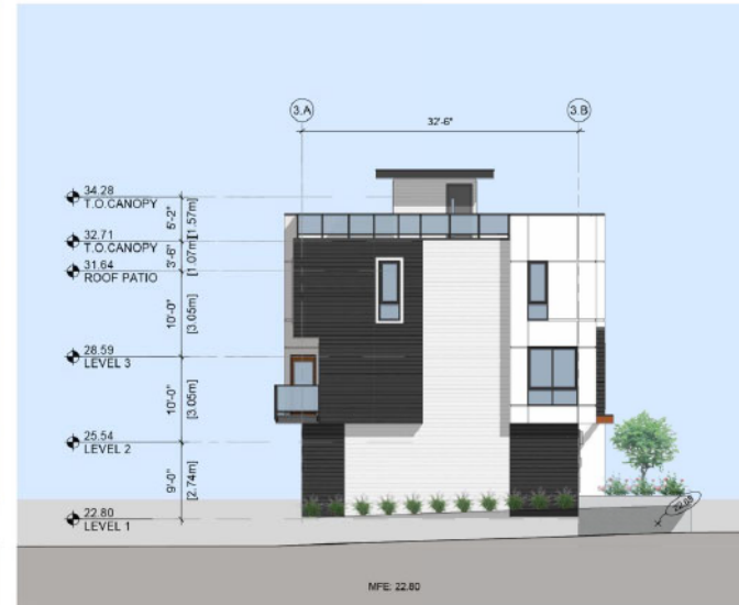
2 BUILDING 3- WEST ELEVATION SCALE: 1/16" = 1'-0"
