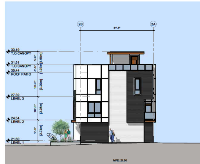
4 BUILDING 2- NORTH ELEVATION SCALE: 1/16" = 1'-0"
