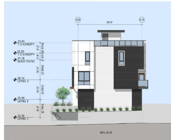
4 BUILDING 3- EAST ELEVATION SCALE: 1/16" = 1'-0"
