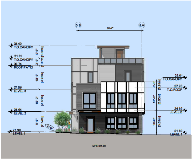
4 BUILDING 4- SOUTH ELEVATION SCALE: 1/16" = 1'-0"
