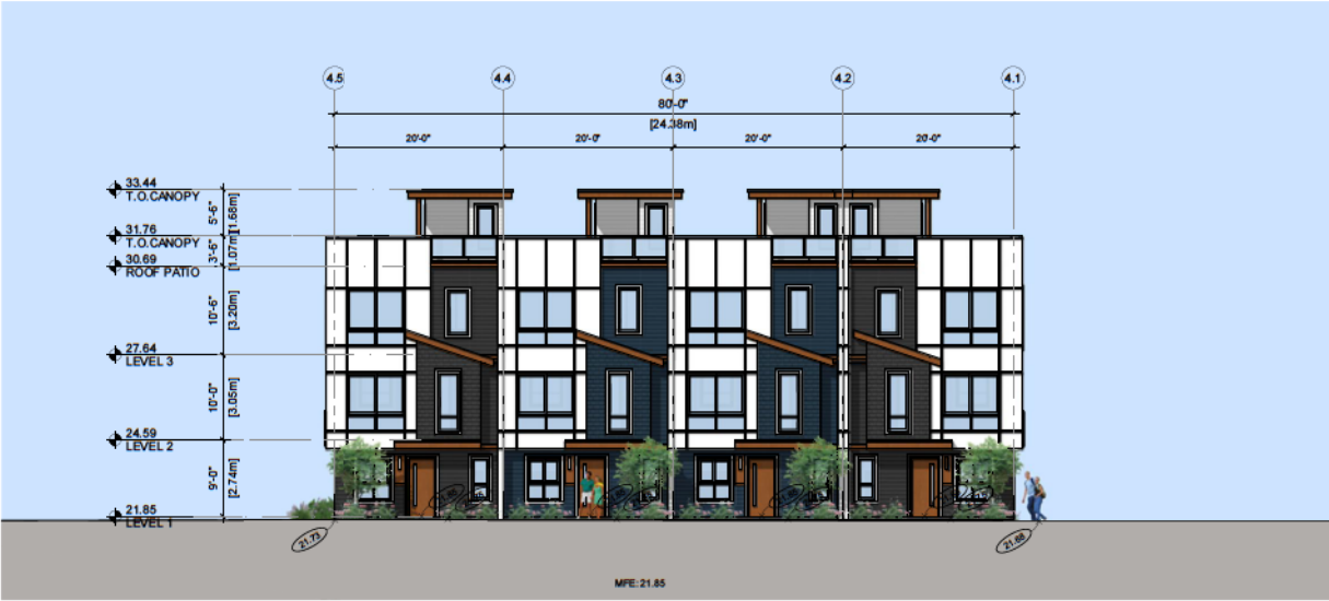
1 BUILDING 5- WEST ELEVATION SCALE: 1/16" = 1'-0"
