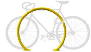
D2 BIKE RACK N.T.S. MANUFACTURER: DEFO PRODUCT: BIKE RACK COLOR: SEVERABLE QUANTITY: 3 OR APPROVED EQUAL
